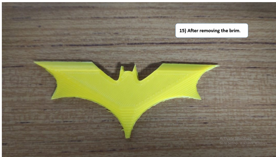
Figure 19: Printed model after cutting the brim.
