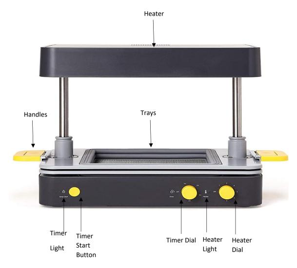
Figure 1 Front view of the Vacuum Forming Machine
